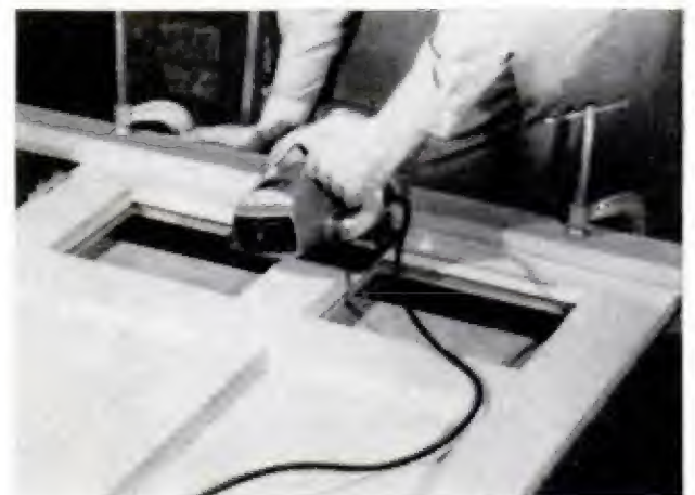
INTERNAL CUT required plunge cut with sabre or circular saw. Use straightedge for the neatest cut
